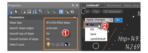
Next, indicate the location of the slope in the drawing. Slope edges can be drawn manually or created from existing drawing lines, depending on the value of the **Specify slope edges** option. The top and bottom of slope can be closed lines.
